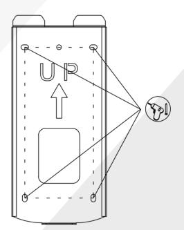
**3** Slot the charging case downwards into the back plate, ensuring a secure fit and tighten with Torx+ Screws provided until secure
