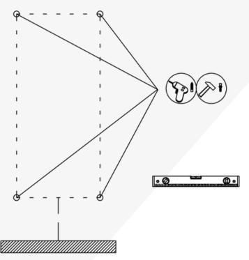
**2** Drill holes accordingly M5\*45mm screws provided with unit using a torque setting of 1Nm fix back plate
